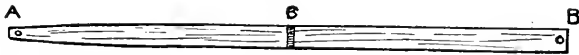
Underside of beam, showing one end shaved down. C. Groove burnt across centre. A.B. Position of hooks.
