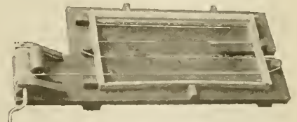
WRIGHT'S FRAME-WIRING DEVICE
