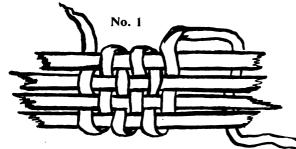
in which the "bams" are put in at the corners, and wherever needed to give a uniform divergence.
