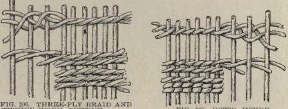
FIG. 206. THREE-PLY BRAT TWINED WORK, OUTSIDE.
