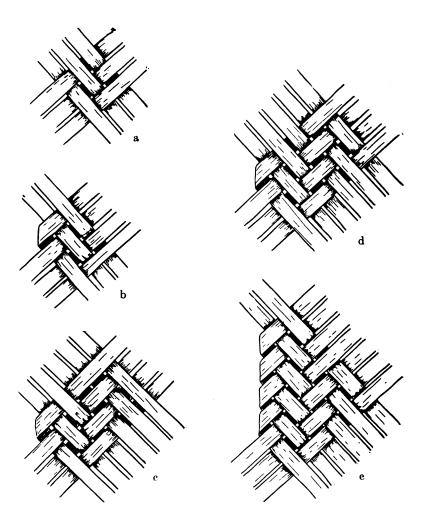
Fig. 16. Method of Plaiting the Headring.
