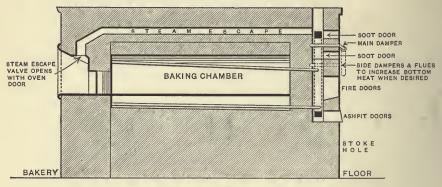
Fig. 208.-Section of Steam-pipe Oven
