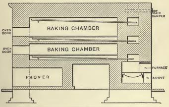
Fig. 212 .-- Hawkins' Patent Regulated Steam-pipe Oven: Section
