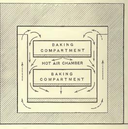
SECTION B. Fig. 203.—Cox's Heat Trap Oven: Section BB (see fig. 202)
