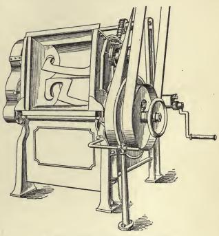
Fig. 218.- "Universal" Kneading Machine, Tilted
