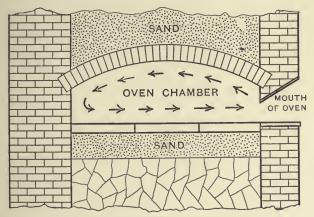
Fig. 195.-Section of Modern Scotch Oven
