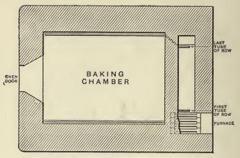
Fig. 211.-Hawkins' Patent Regulated Steam-pipe Oven: Plan
