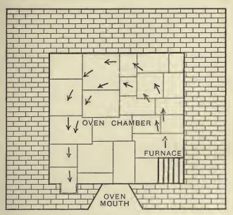
Fig. 194.-Plan of Modern Scotch Oven
