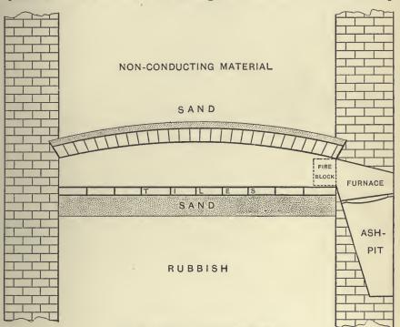
Fig. 199.-Section of Oven through Furnace
