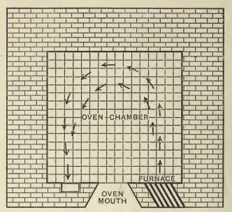
Fig. 197.--Plan of Side-flue Oven
