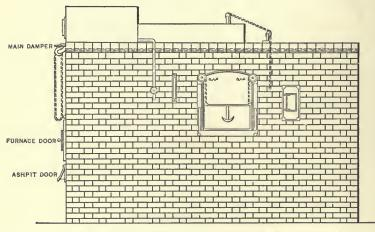
Fig. 216 .-. "Viennara" Patent Steam-pipe Oven: Front Elevation
