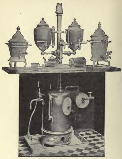
Fig. 183 .- Water Pillar, Coffee-extractor, Milk Urn, and Egg-steamer
