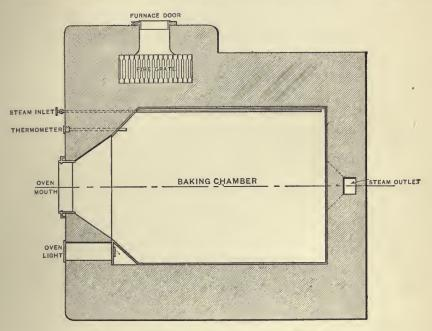
Fig. 214 .- "Viennara" Patent Steam-pipe Oven: Sectional Plan
