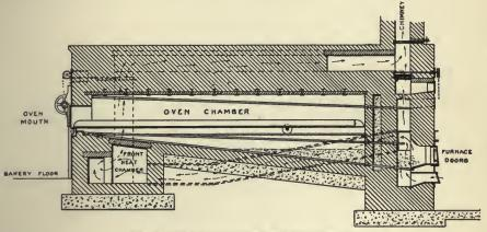
Fig 209.—Baker's Patent Steam-pipe Drawplate Oven
