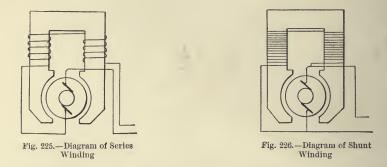
the "compound motor". Each has its advantages and disadvantages, rendering it adaptable to some kinds of work and inadvisable for others. For instance, the shunt motor is best when a constant speed is required at different loads; and the series motor where great starting power is required, as in crane motors, &c. For bakery purposes the shunt motor would seem to be the better adapted on the whole.
