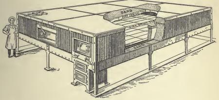
Fig. 201.—Typical American Oven of Flue Type
