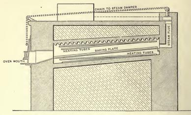
Fig. 215.-" Viennara" Patent Steam-pipe Oven: Longitudinal Section
