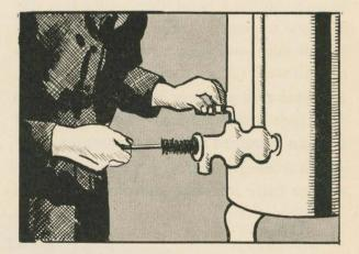
4. Remove clean-out cap at end of the coffee faucet and scrub thoroughly with long, thin brush. Run brush through coffee gauge glass.
