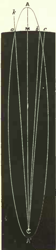
FIG. 155.—Flight of a body projected vertically from the Earth, and regarded as a satellite during its flight.
