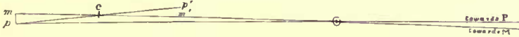
FIG. 15.—Explaining the apparent magnifying of an object or angle by a Galilean Telescope.
