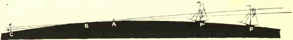
FIG. 51.—Illustrating the effect of changes of Level in shifting the Horizontal Line.
