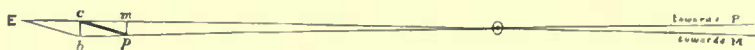
FIG. 17.—Explaining the apparent magnifying of an object or angle by an Astronomical Telescope.
