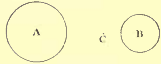
FIG. 470—If A has four times the mass of B , AC = 2 BC .
