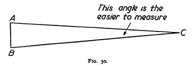
It is also of great importance to make the distance from A to B as large as possible. This is evident because the larger AB the greater the difference between the directions of C becomes, as can be seen by comparing the triangle of Fig. 29 with that of Fig. 30. Now what is the largest distance we can achieve for AB, bearing in mind that A and B must be points that we can actually go to—in order to make the angle measurements of
