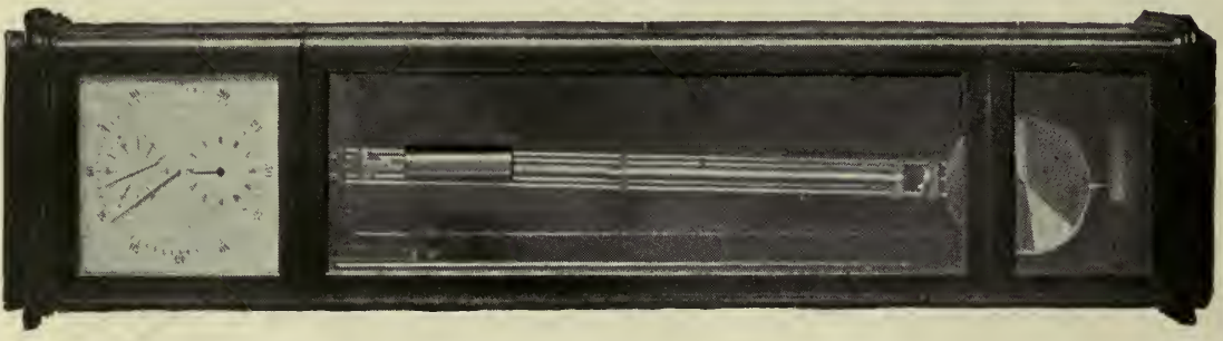
Fig. 48.—Astronomical Pendulum - clock for standard time at the Royal Observatory, Berlin.
