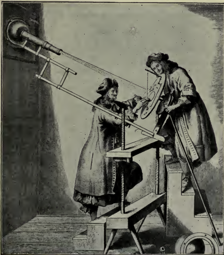
Fig. 129.—Projecting the Sun on to a White Surface.
