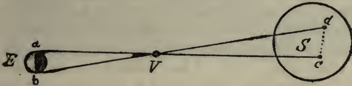
Fig. 150.—Diagram illustrating the measuring of the Sun's Distance during a Transit of Venus.
