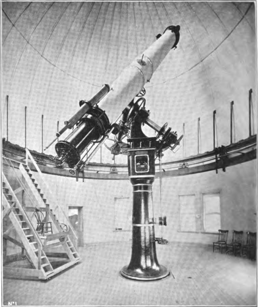
DENVER EQUATORIAL, 20 INCHES APERTURE.
