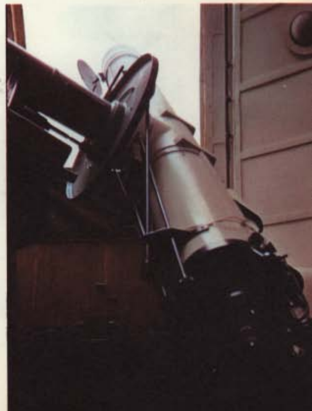
A MODERN REFRACTOR. This is the refractor at the Sternberg Institute in Moscow; the object-glass is 8 inches across. Photograph by Patrick Moore, 1960
