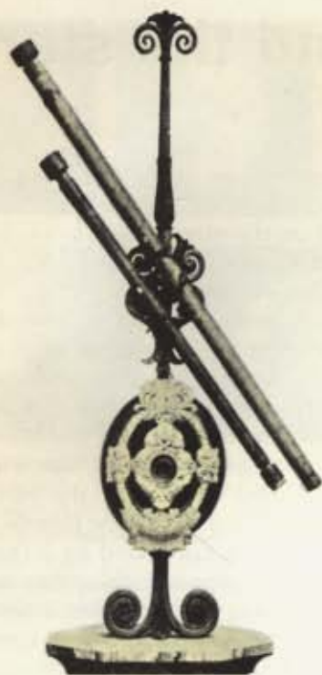
TWO OF GALILEO'S TELESCOPES, preserved in the Tribuna di Galileo in Florence. A broken object-glass, with which the four satellites of Jupiter were discovered, is mounted in the centre of the ivory frame
