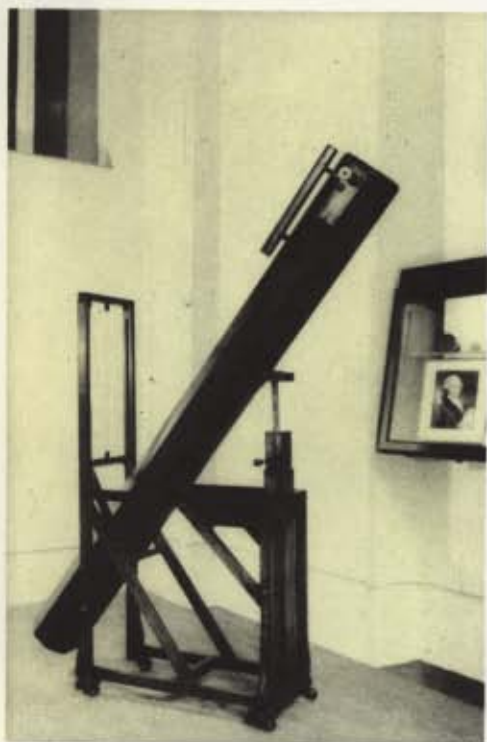
6½-INCH REFLECTOR MADE BY WILLIAM HERSCHEL. This is a replica of the telescope with which Herschel discovered Uranus in 1781
