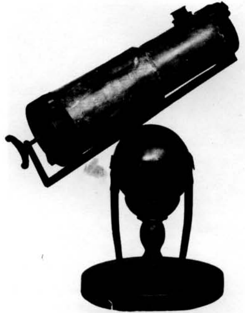
NEWTON'S FIRST REFLECTOR. The photograph shows a replica of the first reflecting telescope, demonstrated by Newton to the Royal Society. The mirror, 1 inch in diameter, was made of speculum metal. Though it was so small, the telescope functioned perfectly, and demonstrated the soundness of Newton's arrangement
