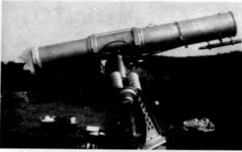
A 12.5-INCH NEWTONIAN REFLECTOR. This photograph shows a typical Newtonian reflector on an equatorial mounting. The focal length is 110 inches. The telescope was used by an English nineteenth-century observer, W. F. Denning, for his studies of planetary surfaces. It is now installed at Henry Brinton's private observatory at Selsey, in Sussex. Photograph by Patrick Moore
