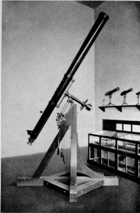
THE TELESCOPE WITH WHICH GALLE AND D'ARREST DISCOVERED NEPTUNE. The telescope was a refractor made by Fraunhofer in 1820
