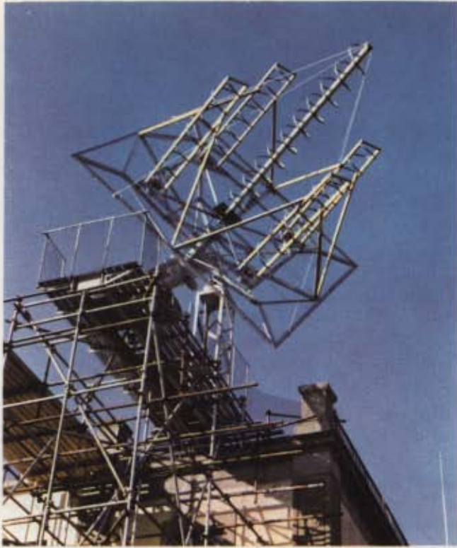
Above left RADIO TELESCOPE AT ARCETRI. One of the Italian radio telescopes, at Arcetri Observatory near Florence. It is entirely different in type from the 'dish' instrument such as the 250-foot paraboloid at Jodrell Bank. Photograph by Colin Ronan, 1961
