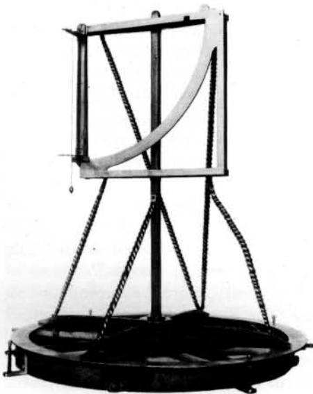
TYCHO BRAHE'S QUADRANT. With instruments of this kind, all built by himself, Tycho drew up his remarkably accurate star catalogue
