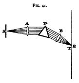
slit, which is supposed to be perpendicular to the plane of the paper. Through this slit a thin line of light passes, and it is this thin line of light which is to be examined in the spectroscope. After passing through s, the light diverges until it falls upon an achromatic lens
