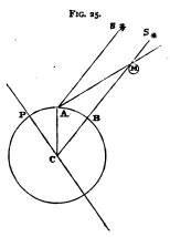
pose, we may suppose to be a sphere. The angle A C B is the excess of the latitude of the station A over the latitude of the station B. This is, of course, known, because the stations are known. Also, since A s is parallel to B s, it follows that the angle AMC is equal to the angle M A S, and therefore the angle AMC is known. In the triangle ACM we therefore know one side,
