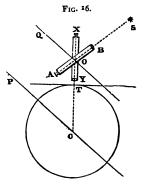
centre of the earth c. In the position AB the telescope is directed towards a star. The angle s o c represents the angle through which the telescope must be turned, in order to be moved from the star to the nadir. Hence the angle  $x \circ s$ , which is the zenith distance of the star, is known.
