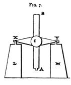
ment may be explained by help of fig. 7. An ordinary telescope, A B, is fixed to an axis at right angles to the telescope. The shape of the axis and the method of attachment of the telescope thereto, are specially designed so as to secure as much rigidity as possible. At the extremities of the axis are pivots,
