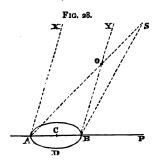
when the earth is at A, we measure the angle S A B. Six months afterwards, when the earth is at B, we can measure the angle S B A. The distance A B is double the distance of the sun from the earth, hence in the triangle S A B we know the base A B, and
