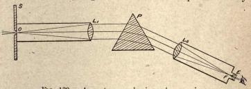
Fig. 139. — A spectroscope having only one prism.
