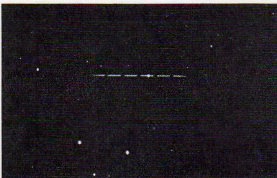
FIG. 22-3 The Baker-Nunn camera (top) on Mt. Haleakala, Hawaii, can detect a 1-foot object thousands of miles in space. To photograph dim satellites, the camera tracks them across the sky, so they appear as sharp dots on the negative (middle). Stars show up on such negatives as long streaks interrupted by the camera's timing device. With the camera stationary, bright satellites become streaks, whereas the stars appear as dots during a short exposure (bottom). This unusual picture shows the Geos satellite on December 20, 1965, with a flash of light reflected from a corner reflector on board the spacecraft (bright dot in fourth streak). (Smithsonian Astrophysical Observatory photo)
