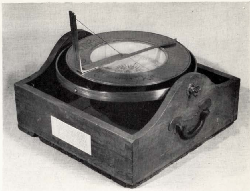
4. Azimuth Compass. English, c. 1720.
