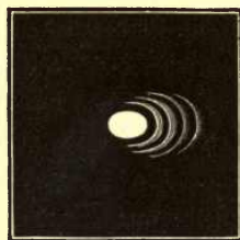
Object-glass not properly adjusted.
