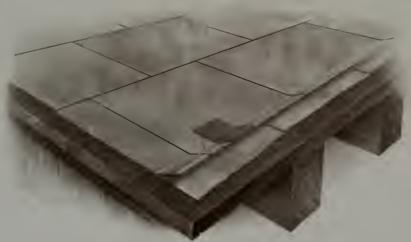
FIG. D.—FLAT-SEAM TIN ROOFING
