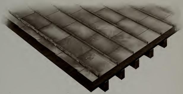
FIG. K.—STANDING-SEAM TIN ROOFING
