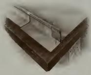
FIG. G.—STANDING-SEAM TIN ROOFING Second operation. Projecting edge turned over.
