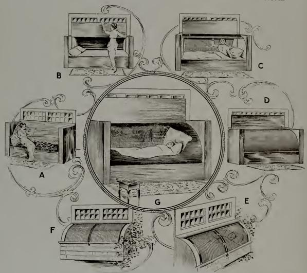
As you will observe from the above Illustrations, about one-third of the CO-RAN FRESH AIR BED is concealed under the seat of a Davenport (A) in the room proper and the rest in an alcove-like addition extending outside about two and one-half feet (F). The dome-shaped wall of the alcove revolves, and by simply swinging it over to the inside (C) the occupant finds himself out in the open, protected by a
