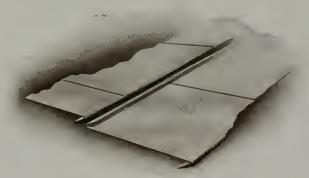
FIG. B.—FLAT-SEAM TIN ROOFING
