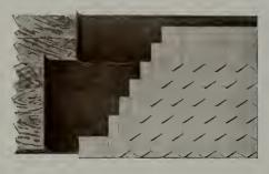
When Xos. 70, 75 and 80 are laid according to the "American" method with a two-inch head-lap over the head of the second course below we have a true hexagonal effect. This style or shaped shingle is applied in many sections for siding as well as roofing and gives a very pleasing "honey-comb" appearance.
