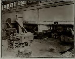
The machine method of making timplate. Only one unskilled operator required to feel the black sheets into the machine. All the processes of tinning, handling and cleaning conducted automatically thereafter, the finished sheets being delivered on the stand shown at the left in the illustration.
