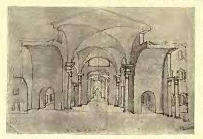
ones had the support of substantial rectangular staircase towers. Pierced ramping buttresses of this kind were employed shortly afterwards, quite likely by the same architect, in the Basilica Nova (Fig. 122), where we get a repetition of the arrangement of Diocletian's Tepidarium, with the great hall of three bays covered by quadripartite vaulting, flanked by six compartments with
