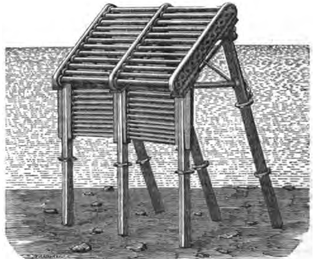
PERSPECTIVE VIEW OF WEBB'S CAST-IRON BREAKWATER.
