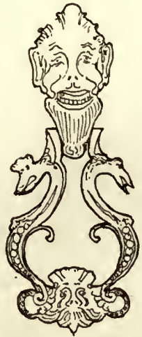
DETAIL OF DOOR KNOCKER SCALE - 3-IN = 1-FT.
