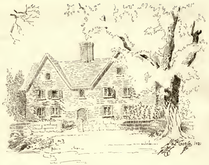
Imaginary restoration, as it may have appeared originally. Drawn directly from photo. Characterless ornament and projecting porch dropped; window-sills raised a few inches; leaded casements substituted for later type; otherwise no alteration has been made in either proportion or detail.
