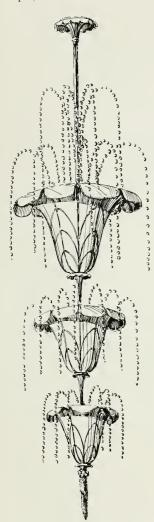
A modern French design done in the manner of Edgar Brandt. The bent glass panels are colored in soft pastel shades. The cut glass beads scintillate in the direct rays of the lamps within the bowls.
