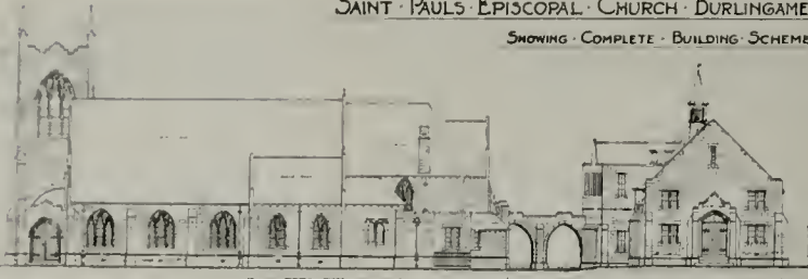
THE FACADE TO OCCIDENTAL AVE. FACING WEST
