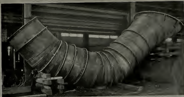
Section of Blue Annealed ARMCO-Ingot Iron discharge pipe made by Downing-ton Iron Works, Downington, Pa., for Calumet Drainage Project, Chicago.
