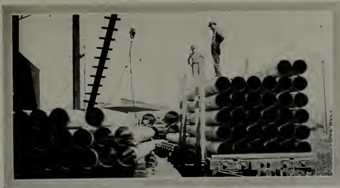
ARMCO-Ingot Iron pipe, 16 to 12 gauge, 6 to 18 inches diameter, manufactured by the Montague Pipe & Steel Company, for the Thermalita Irrigation District, Oroville, California.
