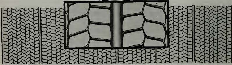
Cross Section of Ideal Rib Lath. Insert above shows actual size of mesh.
