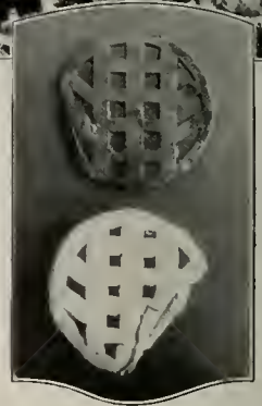
Lead buckle before and after corrosion by the old Dutch process.
