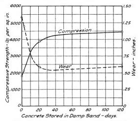
From Bulletin Nº.2 "Effect of Curing Conditions on the Wear and Strength of Concrete" Structural Materials Research Laboratory, Lewis Institute, Chicago, May 1919.
