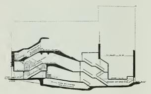
Section (Freeman) showing exit from balcony to alley without losing valuable stage space, and from sides of auditorium through basement tunnel to street.
