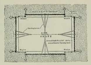
Smoke Vent, Monitor Type, Horizontal Section.
