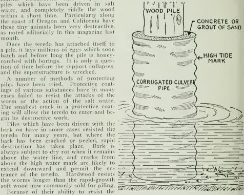
Fig. 2—This drawing shows how corrugated iron pipe may be used to protect pilings from marine woodborers. Note the use of concrete or sand grout to hold the pipe in place.
