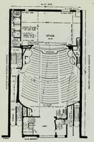
Freeman's suggested plan of aisles and exits, showing exit under stage to alley and incline through basement to street in front.
