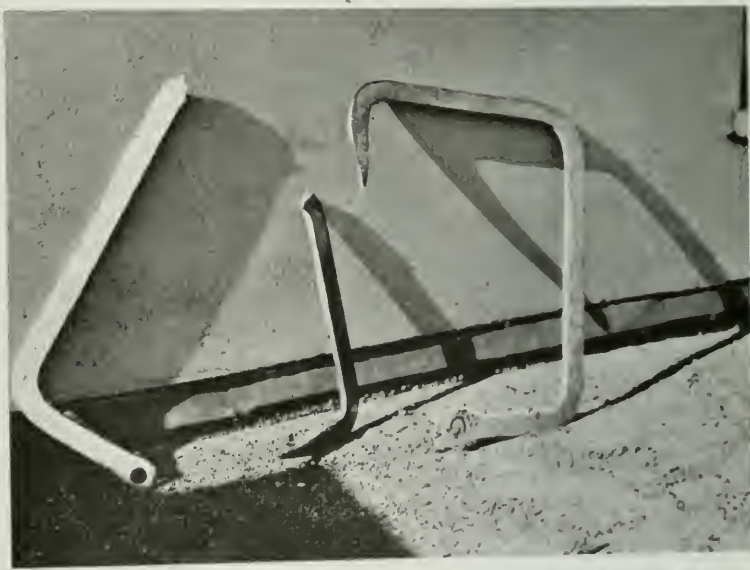
Broken defective hook on the left which killed a worker and temporarily disabled another. The hook on the right was used on the same job and was found inadequate as it failed at a maximum load of 670 pounds.
