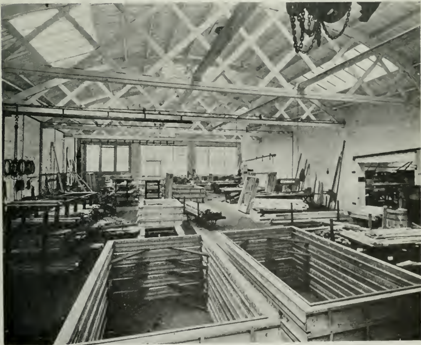
ASSEMBLING SHOP AND SHEET METAL WINDOW DEPARTMENT, UNITED STATES METAL PRODUCTS COMPANY
