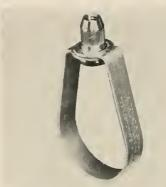
The "Auto-Grip" ring consists of a metal band and a locking insert for attachment to a threaded hanger rod. The insert is self-locking through spring tion as well as through the weight of the pipe supported. Available in zinc or copper plate as standard, for pipe sizes from 1/2 through 31/2 in. Other finishes and metals available on special order. May be safely loaded to 500 lbs. For complete data, write manufacturer, Automatic Sprinkler Corporation of America, Youngstown 1, Ohio.
