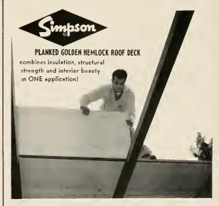
Created for popular exposed beam construction—sturdy roof deck panels made of 1/4" select Western Hemlock Plywood laminated to four layers of 1/2" asphalt-impregnated insulating boards. Panels span 48". Prefinished surface is V-grooved for decorative planked effect. Size: 23" x 96" x 21/4". Check Sweet's Architectural File for full details.
