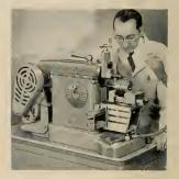
A cam operated piston pump circulates lubricating oil from a large reservoir to all important bearing surfaces. Oil pressure is adjustable and can be maintained at all speeds which cushions the shock of reciprocating ram action and interrupted cuts, resulting in exceptionally smooth and quiet operation even at maximum speeds. Additional information obtainable from the manufacturer.
