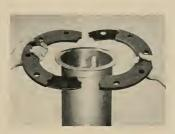
Made of steel, or stainless segments welded into single units, the end leaves of the two halves are interlocked, and when bolted in place, make a positive connection that is stronger yet lighter than is possible with cast iron or forged steel flanges. It is built to A.S.A. specifications for Van Stone flanges at 150 lbs. service and is available in two-inch through thirty-inch tube and pipe sizes. Complete information from Farwell Metal Fabricating, 81 W. Fairfield, St. Paul 7, Minn.
