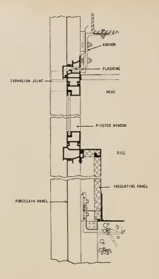
VERTICAL SECTION at left: is through wall showing vertically pivated sash which is reversible for cleaning. Weathertightness is insured by the continuous flashing in the expansion joint at the window head and by designing each horizontal to allow for drainage. Anchors are designed for each adjustment to line, grade and centers and are welded in their final position. Insulating panel runs continuously behind wall diminishing heat loss through mullion.
