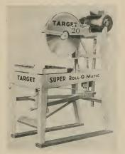
Now a masonry saw user can buy the Target "Super 20" and use it with 14'' blades for cutting brick and tile. Later change to 18'' for refractories or stone, or to 20" blades for block sawing. An outstanding engineering feature is the fact that shaft speed has been scientifically calculated so it is never necessary to change belts or pulleys when switching to a different diameter blade. Just choose the right diameter blade for each job and use it. Additional feature is the "lifetime" Tar-
