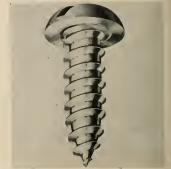
Because of the full thread under the head, considerably more resistance to stripping out is provided than is the case with conventional sheet metal screws whose last thread is not fully formed. Available in Type "A" and "Z" in production quantities in non-countersunk heads. Complete data from Parker-Kalon Division, Clifton, New Jersey.
