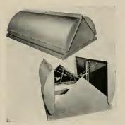
Two double-wall dampers are opened outward by powerful coil springs when a fusible link melts at 212 degree F., creating a roof opening of 28 sq. ft. Projector completely weatherproofed when closed. Can be used for extra ventilation in good weather. Installed singly or in groups. Complete data from the manufacturer The Swarthout Co., 18711 Euclid Ave., Cleveland 12. Ohio.
