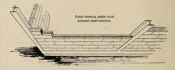
The adobe bricks,  $3\frac{1}{2}$ " x 4" x 16", were fitted directly into the Hsection steel columns. Expanded metal lath was used on every other course of brick to give greater rigidity to the wall. Since the adobe bricks formed non-bearing walls, only a single rather than the usual double course of brick was required. United States Steel vertical columns used were 4"H13#; horizontal beams were 6"WF15.5#. The module was 6 feet, 9 inches.
