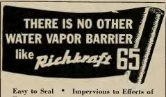
Easy to Seal • Impervious to Effects of Fungi • Lowest-Cost Membrane Capable of Meeting Moisture, Vapor and Fungus Conditions • Made of Two Heavy Kraft Sheets Pre-Treated with Special Fungicides, Bonded With Asphalt
