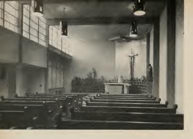
inserts. Major light comes from a series of screened wood panels down each side of the nave in the upper portions of the room plus a large skylight which dramatically lights the chancel area. A part of the floor of the nave slopes forward for better visibility.
