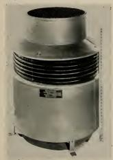
Developed after four years of intensive research and experimentation it uses a sloped circular condensing coil designed to eliminate blind spots common to rectangular coils and permits more efficient drainage of the condensing refrigerant; delivers 100% efficiency which lowers operating costs. Available in 3, 5, 7/2, and 10; 230 volt, 60 cycle single phase motors or 220-208 volt, 60 cycle, three phase motor. Well suited for residential
