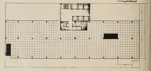
ceiling lighting fixtures, (d) heating and air-conditioning systems in the ceiling. This 4-foot module permits partitions to be installed, removed and reinstalled at any 4-foot point in both directions without affecting lighting, heating or air-conditioning.
