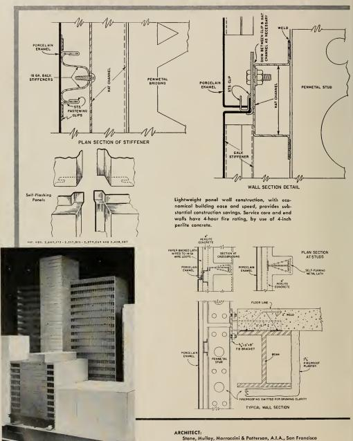
PANEL WALLS of Porceloin Enamel veneer, manufactured and erected by: Architecturol Porcelain Constructors, Oakland
