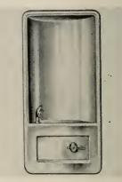
The receptor, weighing less than thirty pounds, is effectively sound insulated and has a convenient removable front access panel. This model provides automatic stream control and a self-closing valve, operated by a chrome plated lever handle. The shielded anti-squirt fountain head is on a raised boss, and is locked to the receptor in a vandal-proof manner.
