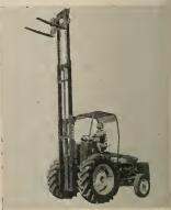
Three models are available for IHC and John Deere wheel and crawler tractors and can be mounted in rear, rear-mounted with operator reversed, or front-mounted. Can maneuver in mud, snow, and pass over chuck holes and clutter; attachments include boom crane, dozer blade, concrete blocktines, snowplow, cement hop-per, personnel platform and bulk materials bucket. Complete data from manufacturer Henry Mfg. Co., Inc., 1700 N. Clay St., Topeka, Kansas.
