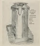
Built of weather-resistant "Aluminized Steel" in exterior construction, and vitreous enameled steel where contact is made with combustion gases. Available in 2 models, Standard 19" square housing, and De Luxe rectangular 19"x34" housing, and any height from 18" to 6'. Mfg. Condensation Engineering Corpn., 3511 W. Potomac Ave., Chicago, Ill.
