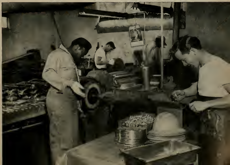
PARTIAL VIEW of polishing room, showing polisher satin-finishing door plate, buffing door framing, pans, small parts, etc.
