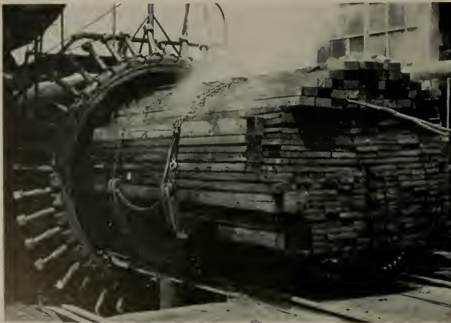
STILL STEAMING — This pressure treated lumber comes from a giant retort at the Baxter & Company processing plant.
