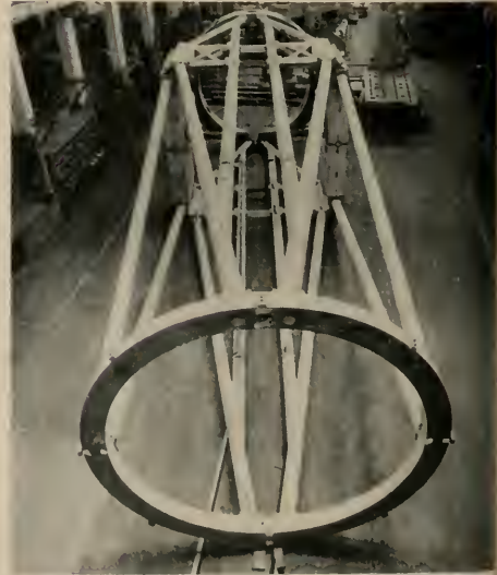
TUBE SECTION ASSEMBLY in shop. Is approximately 43 ft. long and 13 ft. in diameter. Circular ring in foreground will receive the prime focus cage which houses photographic equipment and the astronomer. Circular ring in background will receive the mirror.
