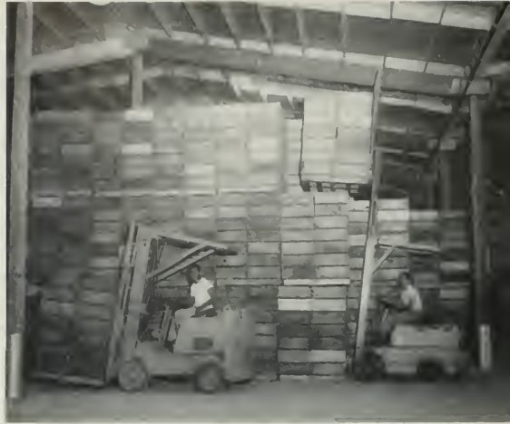
WAREHOUSE IN OPERATION —Designed to store cased canned goods; Shows fork lift trucks stacking green pears which will ripen in the enclosure . . . an ideal method of ripening since the variance of day and night temperature is small due to the thermal qualities of the aluminum roof and siding.
