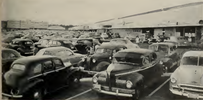
ILLUSTRATION at left shows handicap through lack of walkways. Absence of car stops causes uneven parking and lost space. Two-way traffic creates hazards and congestion. Note: parking lot (rear) entrances from vehicle area.
