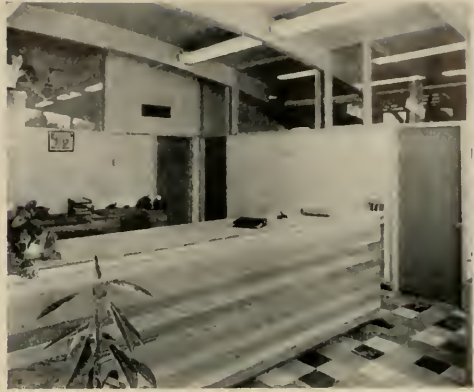
ABOVE —small conference rooms in sales department off lobby. Light supplied by windows above normal wall height in additional space gained by arch roof.
