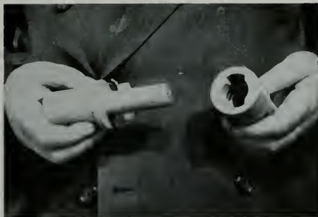
Cast aluminum male and female couplings join tubing ends.
