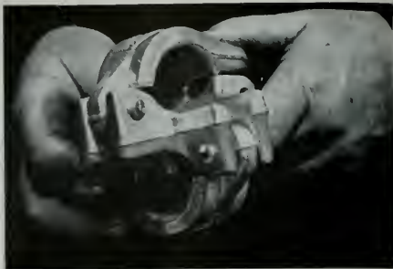
Forged aluminum right angle clamp used to couple horizontal and vertical members.
