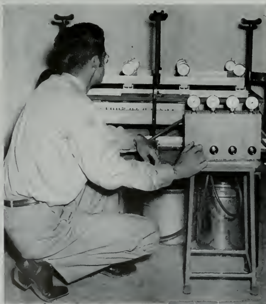
Synthetic, scaled loading of model building units produces stresses corresponding to selected environmental conditions.
