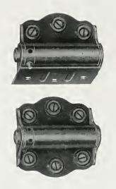
Hinges feature a tension spring easily adjusted to regulate speed of door closing; spring is enclosed in barrel of hinge for protection and attractive appearance. Made of wrought steel; designed for half-surface or full surface applications.
