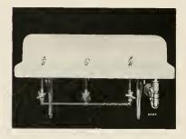
It features the popular Haws "M" head; has an enameled iron recepter with an 8-inch high back; a three-inch full apron and comes equipped with cast iron wall bracket for guick, simple installation. It is particularly adaptable for installation in schools, gymnasiums, large offices, industrial plants and where large numbers of users are served.
