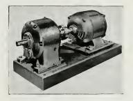
Consisting of a compact, enclosed helical gear drive with separate standard motor, flexibly coupled and mounted on one welded steel base plate. A movable plate between motor feet and welded base plate provides for convenient adjustment.
