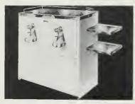
The modern cabinet is of white enamel with stainless steel top, trays and water stations; chrome rail around top protects glossware; top area holds 100 glasses; four side trays hold 20 glasses each; automatic closing, push-back type fill-glass faucets are chromum finished. Capacity five to forty gallons per hour.
