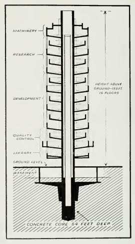
Concrete faundation shown at bottom of abave design is like heavy keel ar anchar to pravide a solid base for tawer—relatively narraw reinforced concrete "stem" cannects base with tower structure proper—each flaar is given cantilever type support from central core. No faundatians directly under walls of square tawer.
