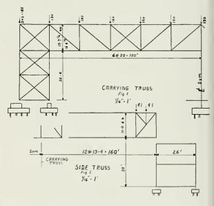
The side trusses, fig. 2 are supported at the outer ends by welded rigid bents. Seismic forces exceeded wind, due to the fact that the bents carried rather heavy floor loads.
