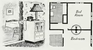
Adjoining rooms where your customers will spend most of their time such as bedrooms or the living room and kitchen -are convenient spots for double outlets. The diagram above illustrates how two outlet boxes may be fastened together ... an excellent arrangement for either portable or fixed telephones.
