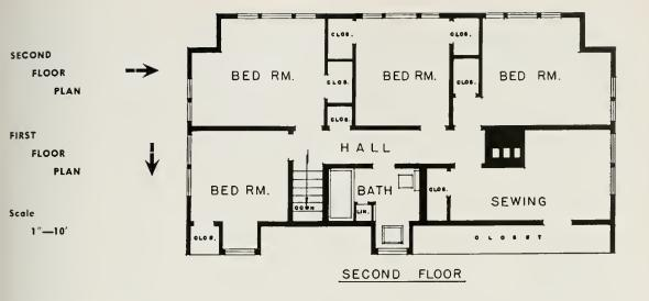
This home is frame construction, one and a half stories with daylight basement. Cedar shingles and cedar siding are used on exterior. Foundation is of concrete. Interiors are of plaster painted or papered. Certain rooms have knotty pine panels. Hardwood floors are used except for Kitchen and Bathrooms which are of linoleum. The roof was left unstained to weather to a natural gray and walls and trim were painted white.
