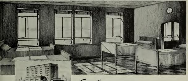
Suggestion: Provide more daylight and better fresh-air ventilation for a ward room in a general hospital with Fencraft Standard Intermediate Combination Windows, such as Type 616 shown here. The sill vent provides excellent ventilation—deflects incoming air upward.
