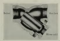
It overcomes back pressure thru a new arrangement of interior surfaces, guiding liquids or gases on a course unobstructed by sharp corners or abrupt changes in path of flow. Strainers are self cleaning, by use of blow-off cock. Suitable for steam pressures up to 50 psi. and temperatures up to 450 degrees F.
