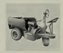
It is built to haul concrete, sand, bricks, motor and other building materials. Runs on airplane type tires and weighs 1000 pounds.
