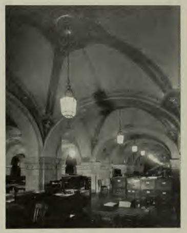
Only scientific air-diffusion could afford proper air-distribution in this room with a vaulted ceiling. Here at the Bank of America, Los Angeles, air enters the room through Anemostats. Lighting fixtures are suspended from each of these air-diffusers.
