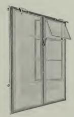
Easily installed from the inside by use of storm sash fasteners, these storm windows are light and provide insulation between the casement unit and the sash panels. Made with double-strength glass and extruded aluminum by Ceco Steel Products Corporation of Chicago, Ill.
