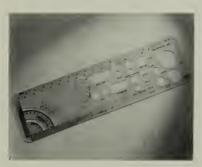
It is made from .030 plastic sheets with printing on negative side to keep it from wearing off. Template is 2¾" x 10"; symbols scaled ¼" to the 1'. Available from Charles Baron, Rapidesign, Inc., P. O. Box 592, Glendale, Calif.
