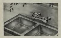
new faucet embodies the same construction found in the ledge-type. Made from brass stampings and precision machined brass fittings, and permanently silver brazed, it combines a unit strength previously unattained in the older style faucets. The long swing spout extends 6½ inches for ample work-
