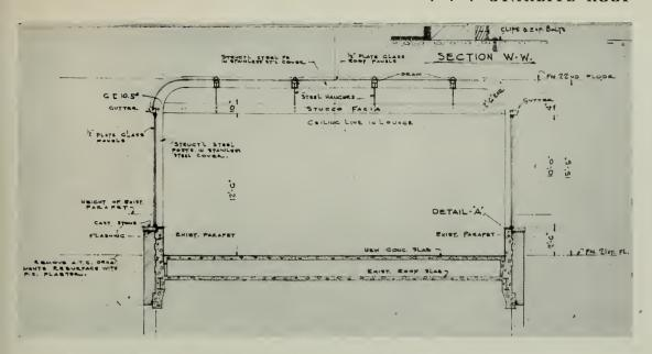
SECTION of the STARLITE ROOF showing changes in walls, concrete cutting sections and installation of over-head and side glass.
