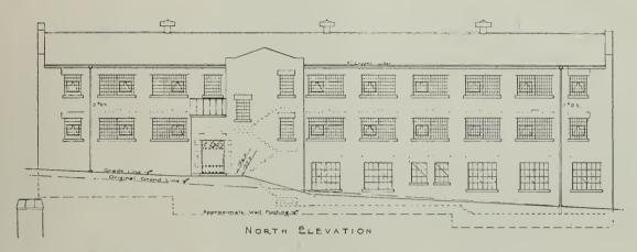
NORTH ELEVATION showing the original ground line, the grade line of the Administration Building and the approximate wall footing.
