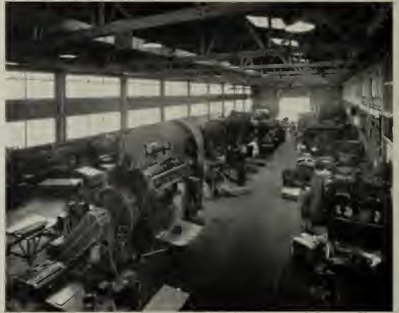
Parts for UTILITY APPLIANCES are die-formed on presses varying up to 375 tons pressure.
