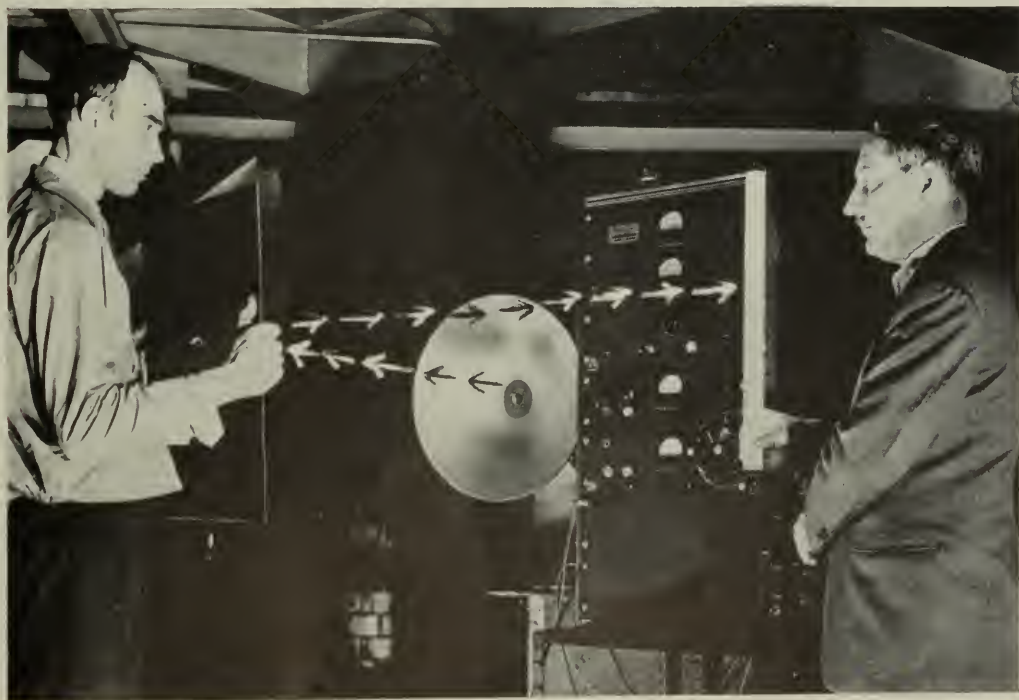
Beamed from the reflector at center to a piece of metal held by the man at left, the waves are deflected back to the fluorescent tube causing it to light with almost normal brilliance although not attached to an electrical circuit. Dotted line indicates path of the radar waves from transmitter to reflector to target. (Westinghouse Photo)
