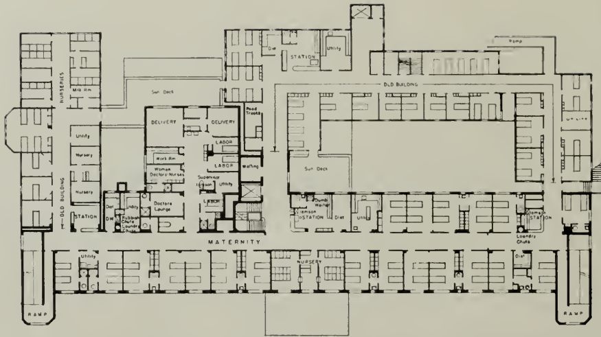
SECOND FLOOR PLAN —Showing Maternity facilities compactly arranged independent of Nursery and rooms; Diet kitchen, nurses' station, and utility.
