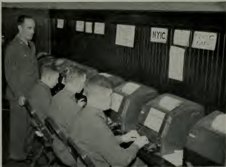
TELETYPEWRITER INSTALLATION FOR INTERCEPTOR COMMAND —Duplicating telephone circuits to a considerable extent, teletypewriters are used for communication with other points on routine matters or when messages of record are desired—as well as providing alternate routes in case of need
