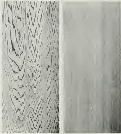
LEFT: FLAT GRAIN WESTERN RED CEDAR SHOWING ITS INTERESTING PATTERN AND THE SHARP CONTRAST BETWEEN THE NARROW DARK SUMMERWOOD AND THE LIGHT SPRINGWOOD IN THE ANNULAR GROWTH RING
