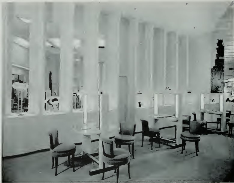
MILLINERY DEPARTMENT, ROOS BROS. STORE, SAN FRANCISCO Note table lighting by means of daylight fluorescent tubes
