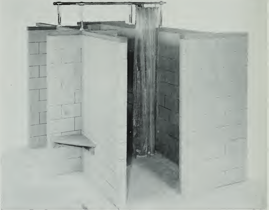
Shower and dressing compartment partitions for Girls' High School Gymnasium, Vallejo, California, as constructed at Kraftite Company plant for tests of structure and seismic resistance. Three-cornered wooden seat in one of the dressing compartments is in Wall B, as tested. At right, is Wall A, as designated in sketch. Hardware for doors, at each end of unit, and plumbing, including shower head, were omitted in test set-up.
