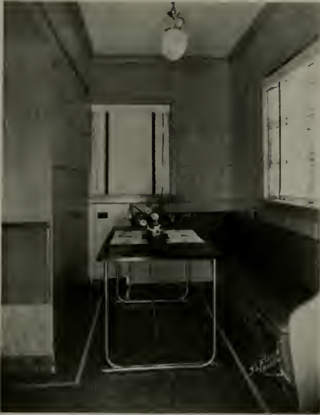
BREAKFAST NOOK, RESIDENCE OF ALDEN BAYLEY, SHELTON, WASHINGTON Walls of Art-Ply, an inlaid plywood
