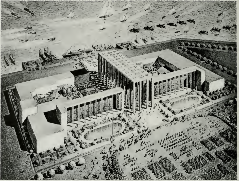
ARCHITECT'S DRAWING OF UNIQUE STRUCTURE TO BE BUILT ON TREASURE ISLAND. OPEN COLONNADE IN CENTER WILL BE 100 FEET HIGH AND 265 FEET LONG. EACH OF THE 48 COLUMNS WILL REPRESENT A STATE
