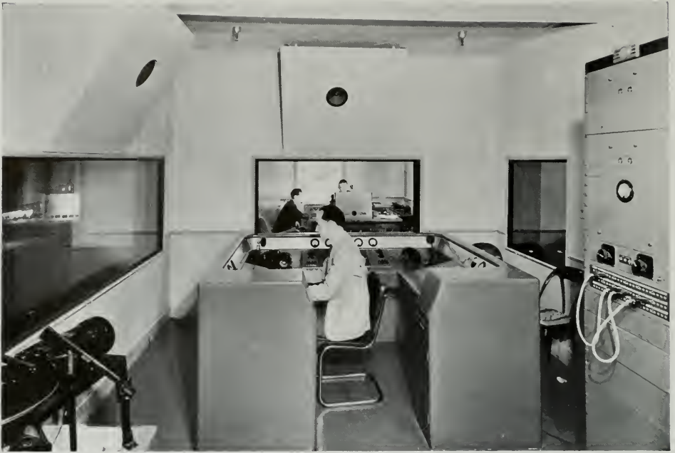
In the foreground is the console of the master control room of Warner Brothers KFWB, with the announcers' studio showing through the glass panel. This room is finished in a grey to match the instrument racks.
