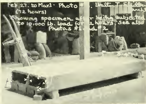
FLEXURE TEST OF FABRICRETE WALL SPECIMEN AS A HOLLOW FLOOR SLAB (Constructed by Method A)
