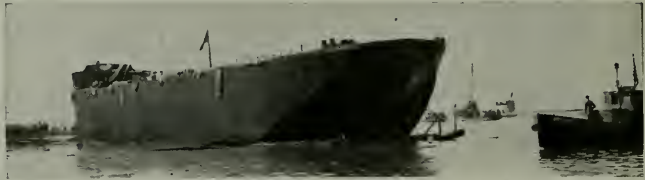
The Concrete Ship "Faith." Length, 336 feet. Beam, 44 feet. Capacity 5,000 tons. San Francisco Shipbuilding Co., Builders
