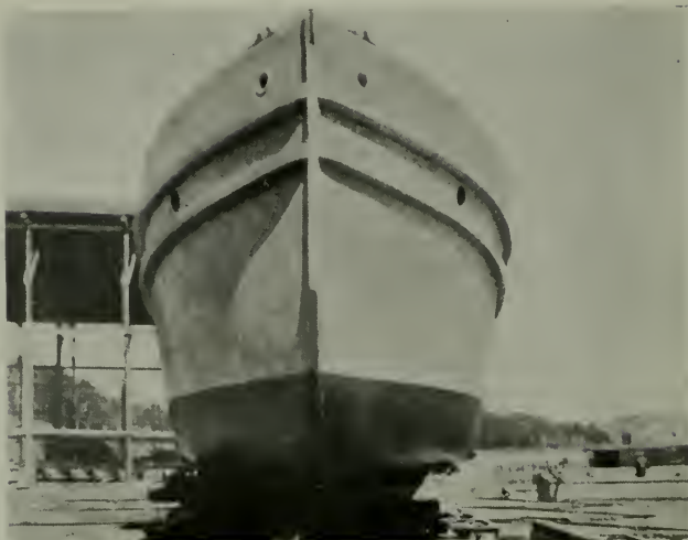
CONCRETE SEA-GOING VESSEL FOR COASTWISE TRAFFIC IN SCANDINAVIAN WATERS
