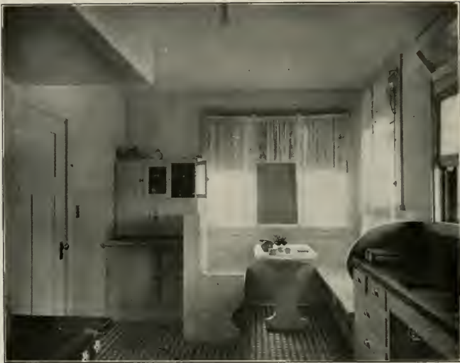
Kitchen in Mr. Reddell's Home, 2578 Buena Vista Avenue, Berkeley, showing treatment of kitchen with Hoosier cabinet installed, "Fullman" breakfast room in connection. Note the convenient arrangement of gas range (with overhanging hood) in relation to sink and kitchen cabinet.
