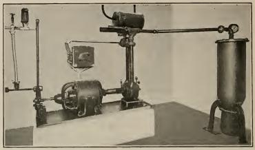
Combination Jarvis Oil Burner and Vacuum Sweeper
