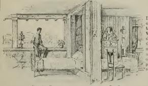
Isometric view of the Oscillating Portal Wall Bed showing how the same bed may be used, at will, either on the sleeping porch or in the room.
