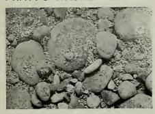
Here is a photograph of the PRATT BUILDING MATERIAL CO'S. (C. F. Pratt, Pres.), washed concrete gravel ranging in size from 0 up to 1½ inches. There is 36% of washed sand from 0 to 3\$ 25% of crushed rock and 45% of gravel from 38 to 1½ inches. We absolutely guarantee not over 21% of voids, just enough space for the cement and water. Douglas 300—easy to remember — will give you additional information. Our office is in the Examiner Building.
