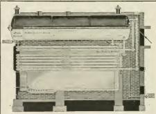
WITH many tubes in one header, the unequal expansion causes leaky joints. Rerolling thins the tube ends and means new tubes. In the design of a header holding but two tube ends each tube can expand without strain on header or joints. This is another feature of the
