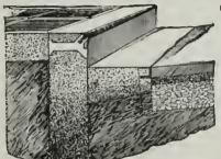
GALVANIZED STEEL CORNER BAR Prevents Chipping or Breaking on Edges
