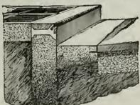
GALVANIZED STEEL CORNER BAR Prevents Chipping or Breaking on Edges
