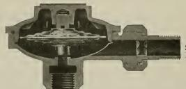
Sectional view of the Dunham Radiator Steam Trap.
