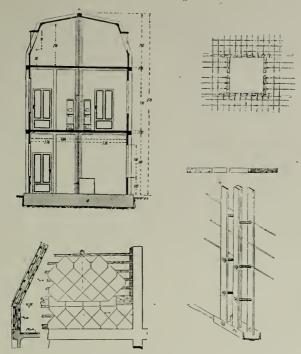
Figure 3 (left top) shows section of Building shown in Fig. 2. Fig. 4 (bottom right) is detail of Wall and B indow Opening. Figure 5 (bottom left) is a detail of the Roof Construction
