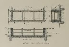
between the boxes before the bottom has hardened with fresh concrete of the same consistency as previously made, tamping thoroughly and working near the boards with a paddle-shaped stick to bring the finer material to the front.
